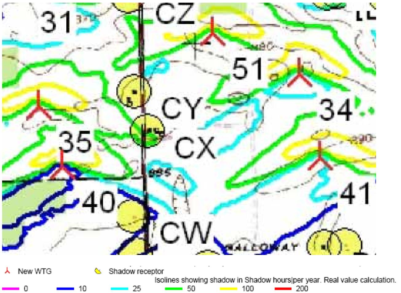
**Figure 3: Graphical Description of WindPro Predicted Shadow Flicker Impact Isolines Surrounding Maximum Impact Receptor (in Shadow Hours per Year)**
